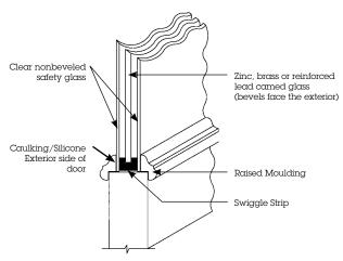
\*For many people, bright zinc and brass caming do not satisfy their particular esthetic requirements. Therefore, PINECREST® offers an alternative reinforced lead caming which has the look of lead and the structural integrity of zinc or brass. There is an extra charge for brass reinforced lead caming.
